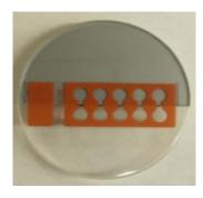
Fig. 4. Placement of test slide on petri dish so that the median line aligned with the edge of the tape.
